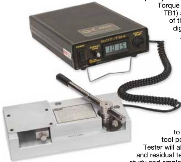
This one tester will provide all the information that previously required two separate testers, and increased consumption of Safe-T-Cable® for verification of application tools. A single installed cable assembly can first be tested for minimum load – hold (flex limit test), and then be tested to destruct load (optimum tool performance). The SCT-TB4 Tester will also provide applied tension and residual tension data for engineering study and employee training purposes.
