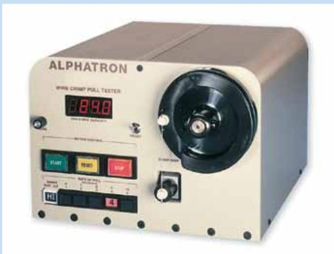
The MPT-250B-SC Motorized Pull Tester is designed to perform pull-off testing of .020, .032 and .040 diameter sizes of Safe-T-Cable® to verify compliance requirements of SAE Aerospace Standard AS4536.
