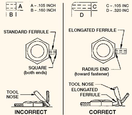
**FIGURE 7: Low Profile Application For .022, .032 and .040 Inch Safe-T-Cable®**
