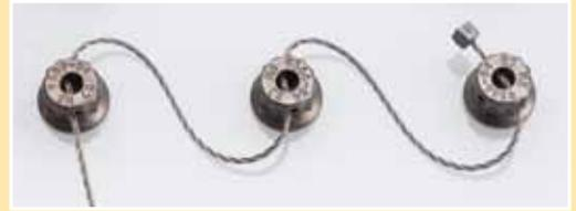
A Cable Assembly is threaded through the fasteners in a direction which will exert a positive or neutral pull when tension is applied.
