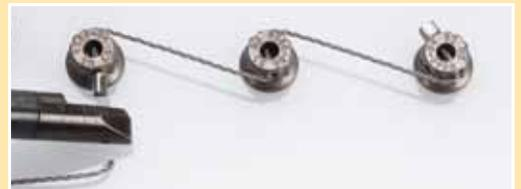
The ferrule is firmly crimped, and the cable is cut flush with the end of the ferrule.
