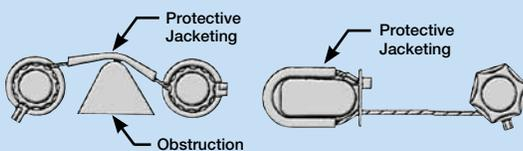
**SAFE-T-CABLE® JACKETING FOR PROTECTION.** It is recommended that a tubular jacket be placed over Safe-T-Cable® when it is installed in an area where it will be in contact with obstructions or surfaces that may damage the Safe-T-Cable®. The tubular jacket material shall be capable of meeting the temperature range of the application. It shall also be resistant to oil, and chemical environments.
