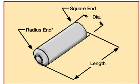
**A Special Elongated Ferrule** is available for those installations. The longer reach of the ferrule provides a stand off to the tool nose. Combine that with the radius on the end next to the fastener (radius not required on the F10-08 .022 elongated ferrules due to the small outside diameter). The radius allows the ferrule to be installed at an angle without loss of tension on the cable when the ferrule returns to the straight position.
